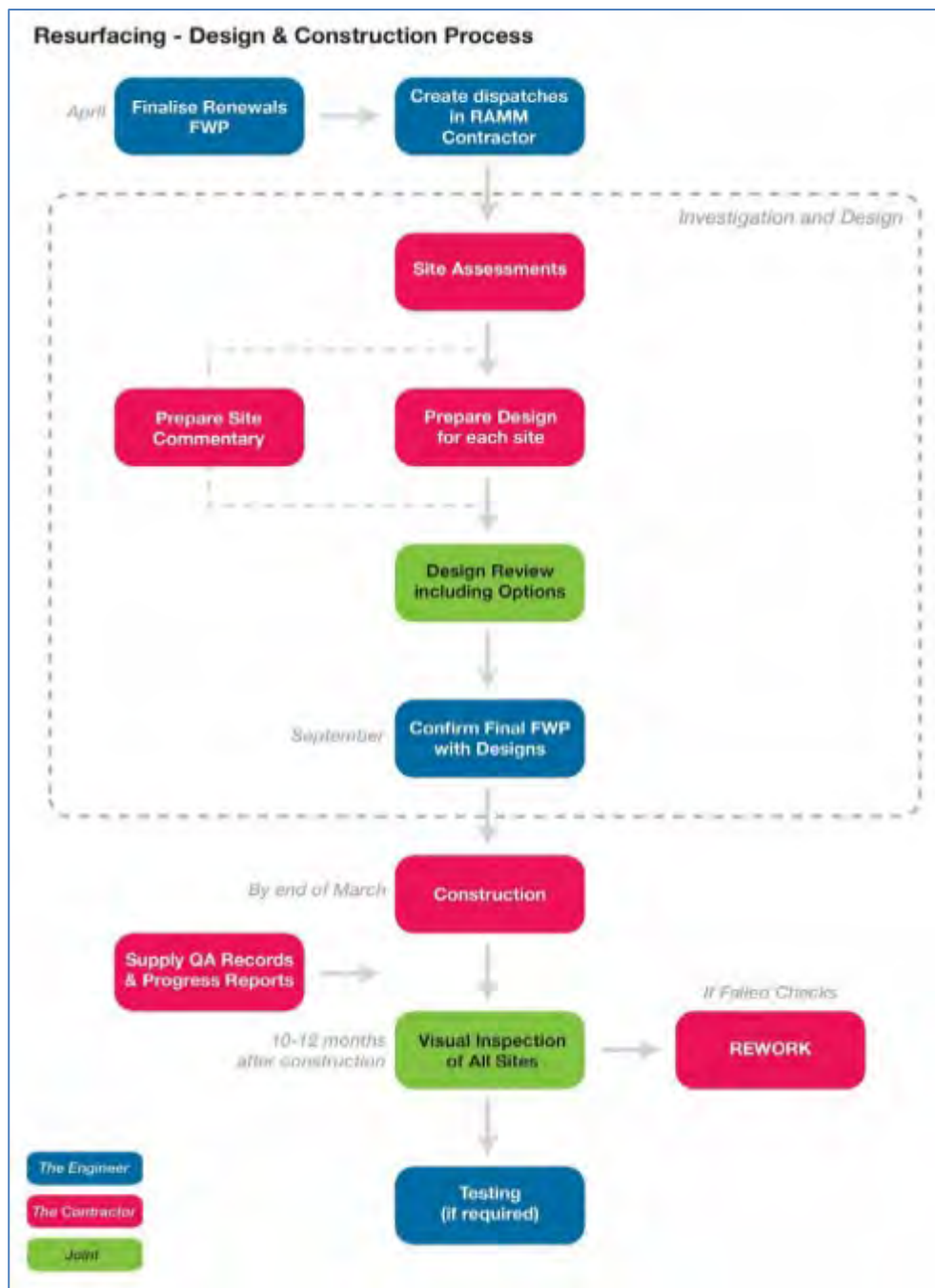
Figure 7-7: Resurfacing Design & Construction Process
